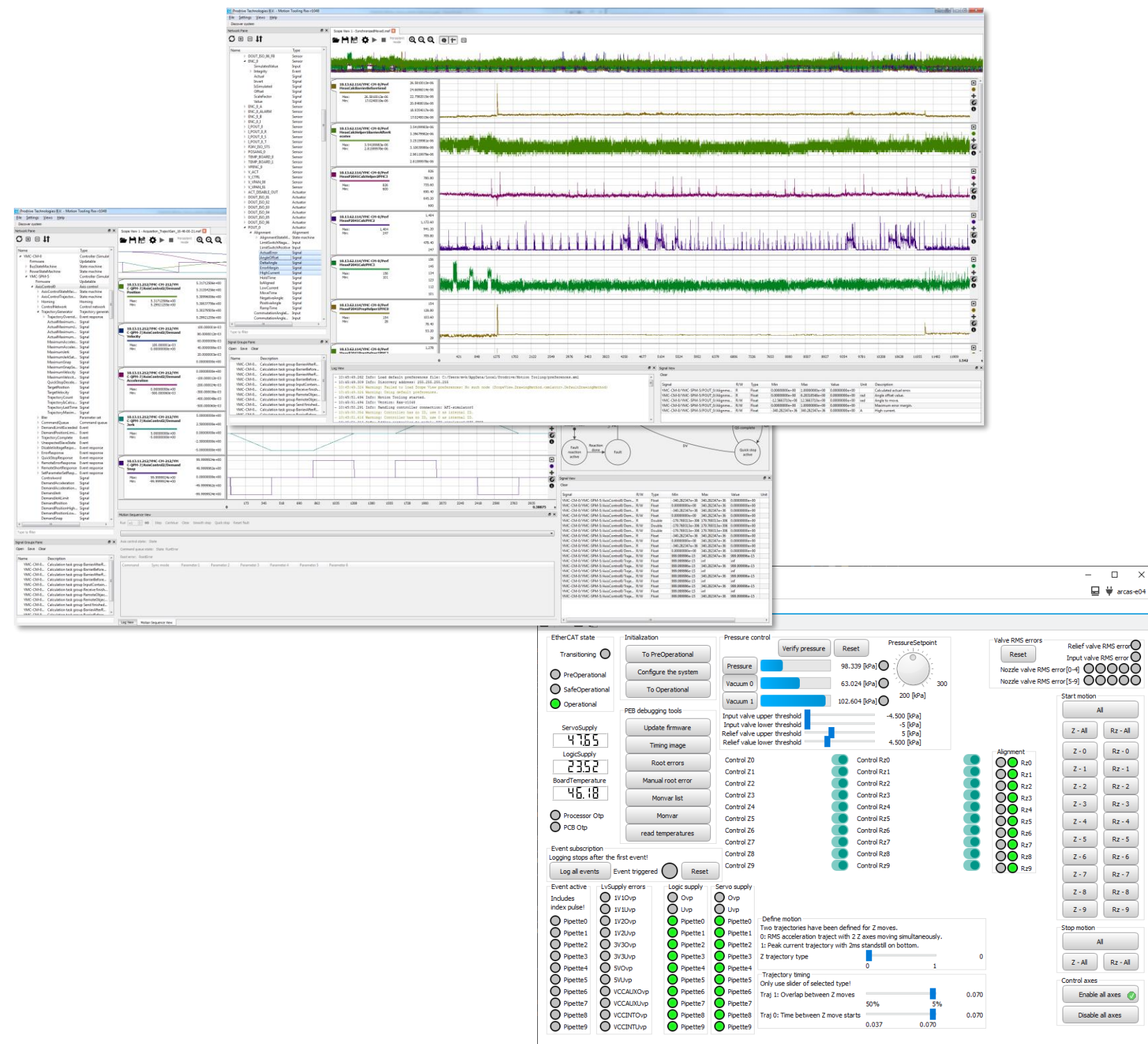
PMP motion tooling, showing the signal acquisition and HMI-views
